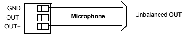
FIG. 5 Wiring the rear AUDIO IN and MIC OUT for use with Unbalanced Audio
